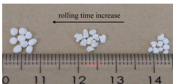
Fig. 7. Morphology change of the \text{Li}_2\text{TiO}_3 pebble by dry-rolling granulation process.
